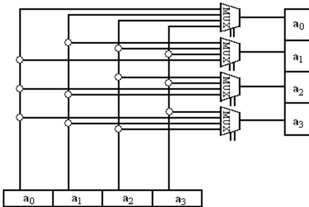
**Figure 3.** The rotation operation (ROTR) implementation using multiplexers
