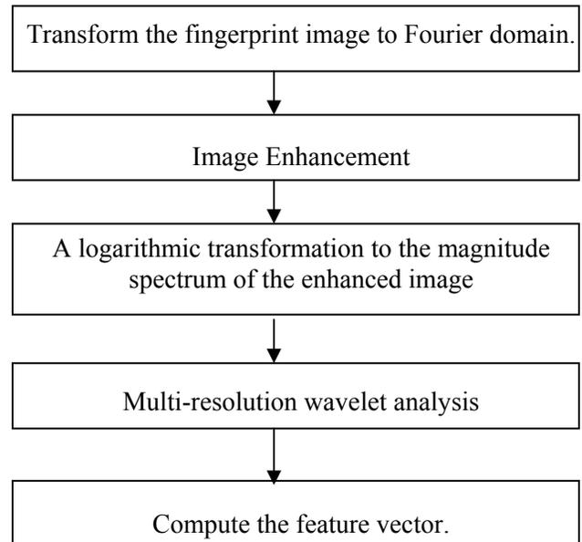
**Figure 2:** Feature extraction block diagram
