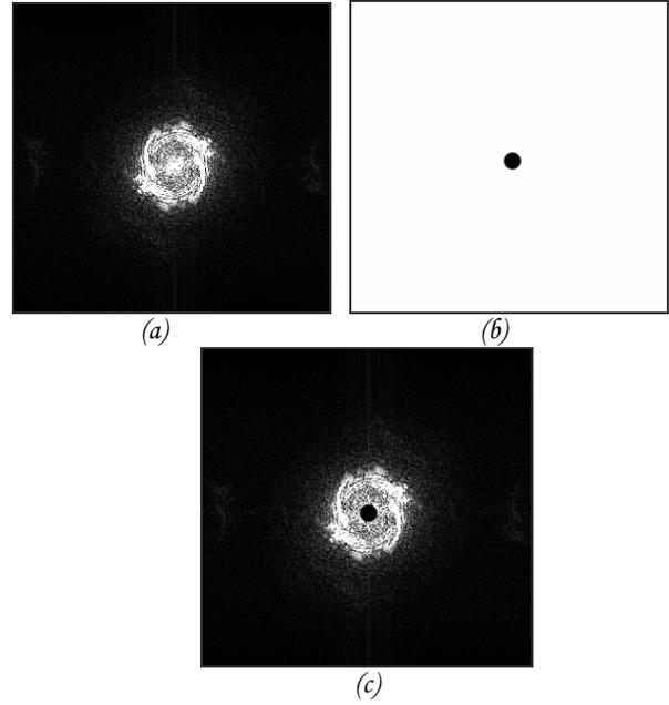
**Figure 3:** How Images are filtered in the frequency domain
