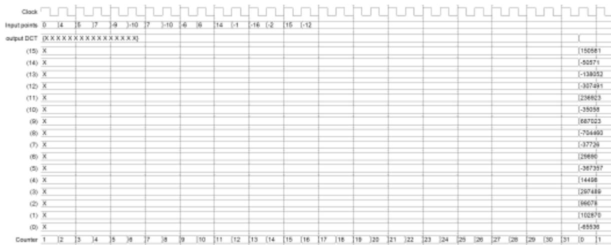
Figure 5: Simulation of the 16-point DCT
