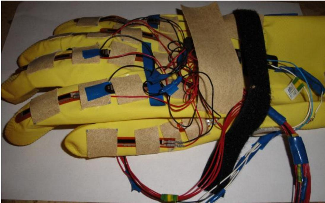
**Figure 1** The data-glove with the finger and wrist mounted sensors
