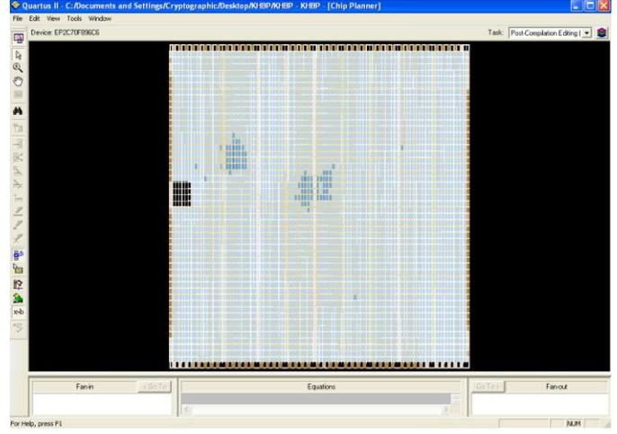
Figure 8. Floor-plan of power based key hopping implementation
